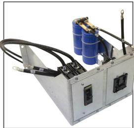
Output filtering is essential whenever there is need for low AC ripple and low noise on the DC bus for critical loads. The standard DC output filtering limits ripple to no more than 30mV RMS on 12, 24 & 48Vdc units, and 100mV RMS on 130Vdc units, measured at the battery terminals. This feature meets the specifications of NEMA standard PE5-1996, and is recommended for installations using Valve Regulated Lead Acid (VRLA) or gelled electrolyte batteries.
