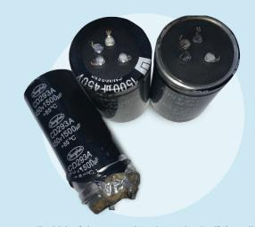
Can you tell which of these capacitors is good or bad? Actually, all three have failed and need to be replaced.
