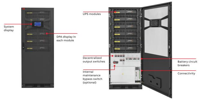
Each high-reliability, standardized module is self-contained and can be swapped at any time, so nothing has to be ever switched off – making routine maintenance safe and easy. Conceptpower DPA 120 is designed to secure continuity of critical operations for small to mid-sized data centers, server rooms and other IT applications. It also protects industrial automation processes, healthcare facilities and many other vertical markets where operations are of a critical nature.
