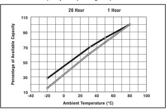
Capacity vs. Operating Temperatures: Above are the changes in capacity for wider ambient temperature range, giving the available capacity, as a percentage of the rated capacity, at different ambient temperatures. The curves show the behavior of the battery after a number of cycles.
