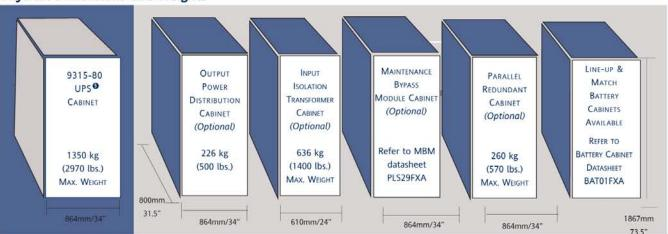
All accessories feature plug and play capability. Shipping pallet and packaging adds 50 to 300 lbs. per shipping unit. Casters are standard for ease of installation.
