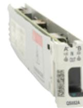
Downstream input units require +/- 190Vdc (+/-188Vdc to +/-192Vdc) nominal input via RJ-21 connected twisted pair copper lines. Each QS882A downstream converter has a maximum input current limit at 0.251A per channel. Downstream output units provide -54.5Vdc (-52Vdc to -54.5Vdc) output via a pluggable connection. Each QS882A downstream converter unit will deliver 65 Watts per channel.
