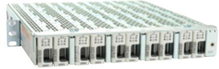
The Line Power System downstream shelves are easy to setup and operate. All shelf options are equipped with 25 pair input cables terminated in an AMP/Champ RJ-21 connector for easy connectivity. The -48Vdc output is through a Molex Minifit SR connector and an interface cable is included. When an optional fan tray is added, the power interface cable is also included.
